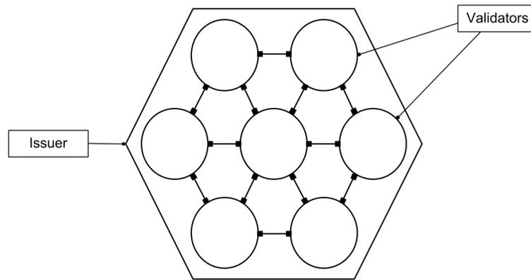
Figure 1 shows a decentralized model in which the validators are separate entities from the issuer and in which validators use distributed consensus to synchronize their ledgers. It would also be possible to have an internal construction for a cell which was more centralized where the issuer also undertook the validation of transactions and maintenance of the ledger.
